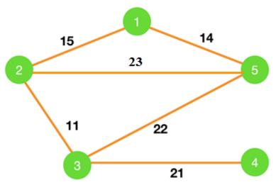
Which of the following edges form the MST of the given graph using Prim'a algorithm, starting from vertex 4.
